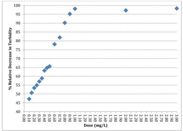
Figure 5. 5: Equilibrium percentage relative decrease in Turbidity as a function of dose of Ferric chloride.
