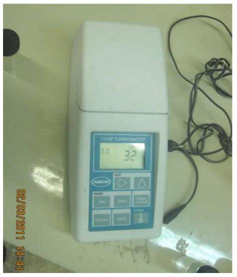
Figure 4. 4: HACH Turbidimeter used in IEWS lab.
